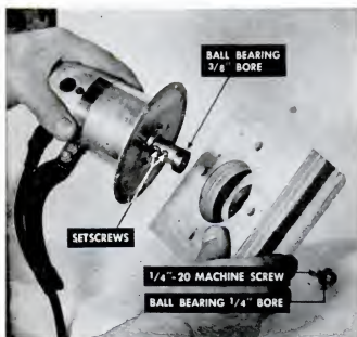
The \frac{3}{8} " ball bearing on eccentric slips into steel disk fastened to movable block. Disk is just visible through hole in motor block.
